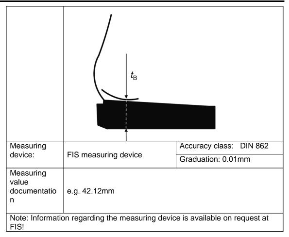
Note: The overall standing height of the athlete is the sum of bearing surface height and the height of the ski boot soles. However the overall standing height is not specified as independent parameter, instead the individual specifications for bearing surface height and thickness of the ski boot soles apply.
